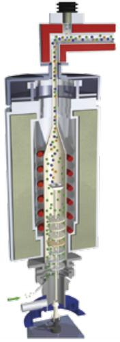
Natural vertical gas flow through the STA furnace to the heated adapter with capillary inlet and bypass
